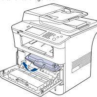
3. Thoroughly roll the cartridge five or six times to distribute the toner evenly inside the cartridge.
